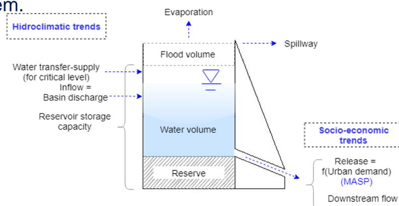
Figure 2. Conceptual model of a single reservoir.
